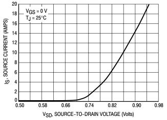
Figure 9. Diode Forward Voltage versus Current
