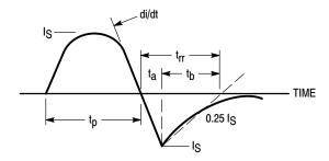
Figure 14. Diode Reverse Recovery Waveform
